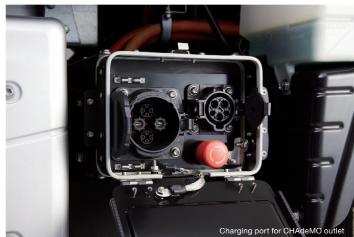
Charging port for CHAdeMO outlet
